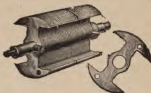
FIG. 95.—Core of a magneto-generator armature, and end view of same. The insulated wire is wound on from end to end, parallel to the spindle and almost to the top of the flanges at either side, which are left bare. The form of core here shown is "laminated," or composed of a number of pieces, as indicated by lines running across the axis. This improvement was introduced by the Holtzer-Cabot Electric Co., and has the advantage of permitting a more accurate adjustment, a greatly enlarged field, and consequent increase in output of power.
